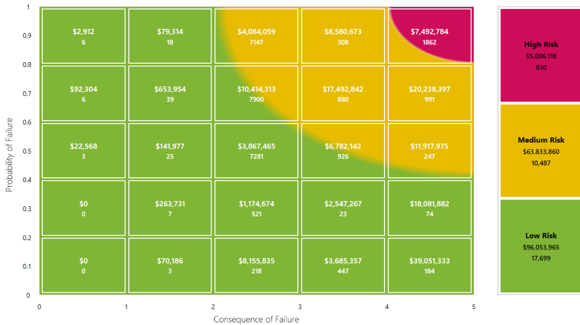
Figure 1-9 Building Management System Risk Matrix
